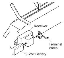
Figure 15 - Installing 9-Volt Battery In Receiver
